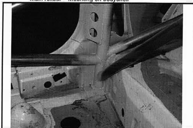
SC-12) Arceau principal – Ancrage sur la coque Main rollbar – Mounting on bodyshell
